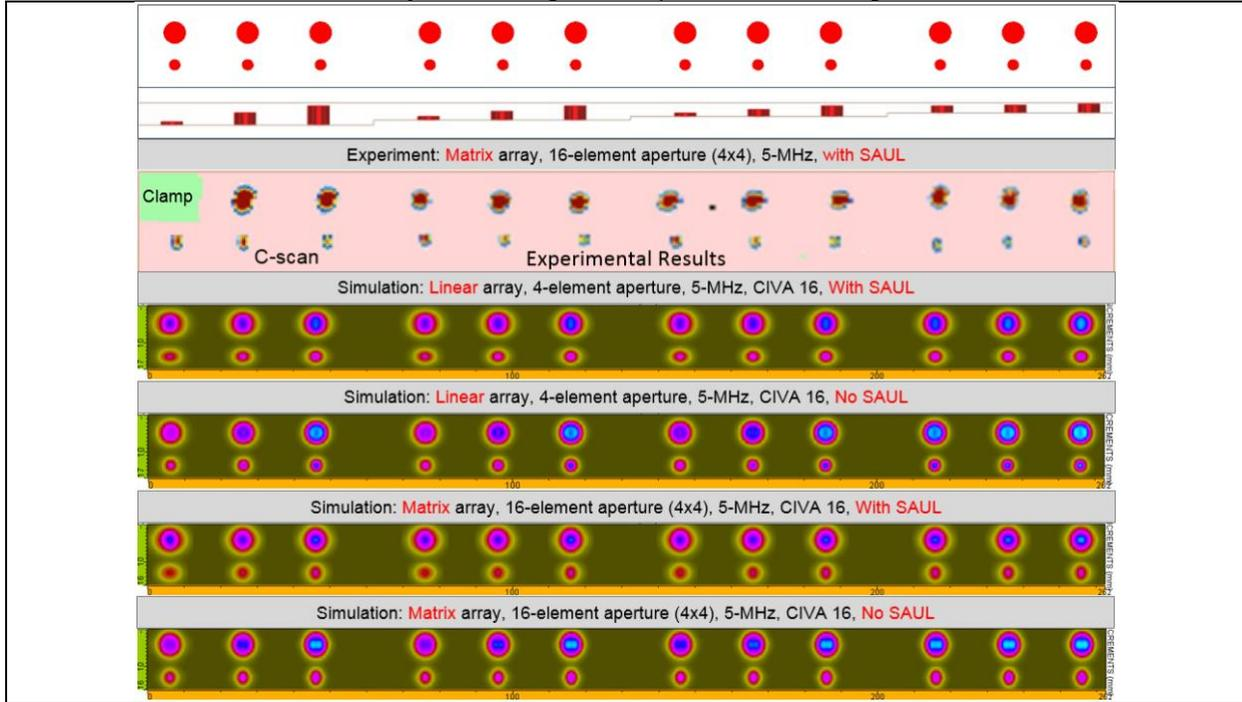
Figure 9. Simulation results are shown for the flat section of the composite calibration block to allow simulation and experimental results to be compared with respect to detection, sizing resolution, and relative signal amplitudes. The results shown here are for 5 MHz linear and matrix probes with 4 elements active (linear) and a 16-element aperture (4x4) for the matrix probe. The indications were sized and are compared in Fig. 10.
