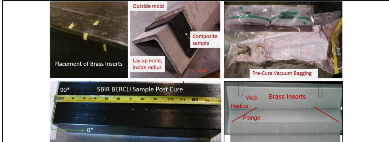
Figure 3. Steps in fabricating test specimens with embedded defects: placement of inserts at three depths in laminate; vacuum bagging and autoclave cure. Radiographic imaging was performed to confirm the location of the brass defects.
