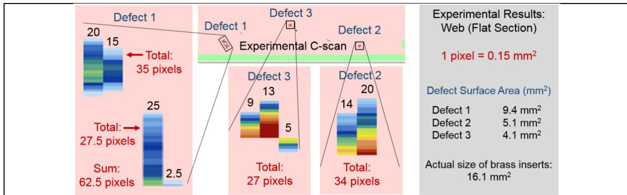
Figure 4. Experimental UT results in the web (flat) region of the test specimen with brass inserts (see Fig. 3).
