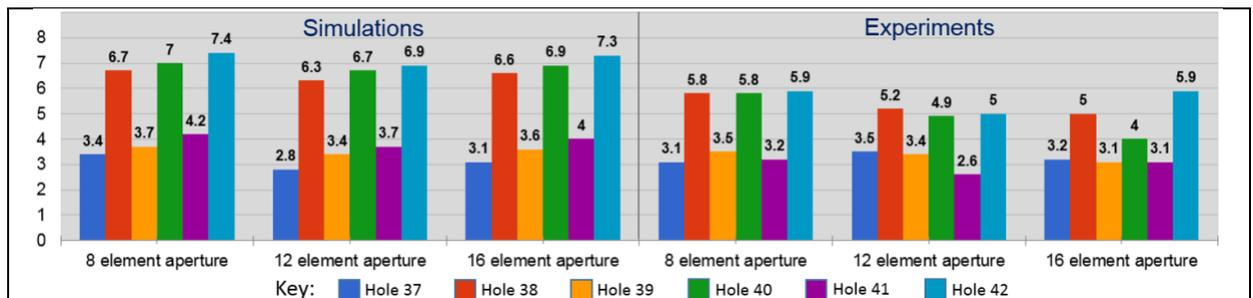
Figure 13. Bar charts showing hole diameters estimated from simulations (left-hand side) and experiments (right-hand side) using SAUL for the convex radius for 3 reception apertures (8, 12 and 16 elements). Actual diameters are 3 and 6 mm.
