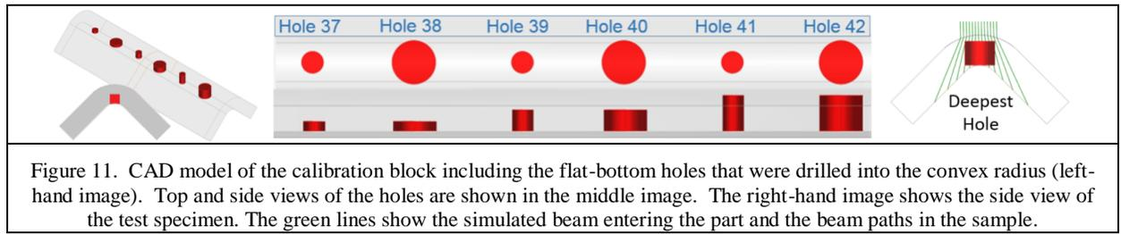
Figure 11. CAD model of the calibration block including the flat-bottom holes that were drilled into the convex radius (left-hand image). Top and side views of the holes are shown in the middle image. The right-hand image shows the side view of the test specimen. The green lines show the simulated beam entering the part and the beam paths in the sample.
