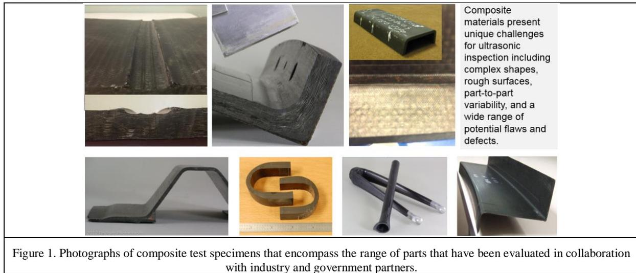
Figure 1. Photographs of composite test specimens that encompass the range of parts that have been evaluated in collaboration with industry and government partners.
