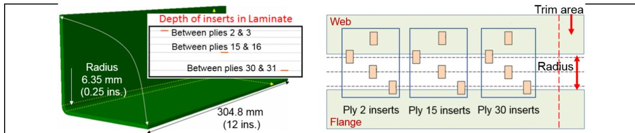
Figure 2. Schematic diagrams showing the CAD model for composite test specimens (left-hand image) and the location of embedded inserts at three depths in the laminate. The samples include a trim area that is available for porosity measurements.
