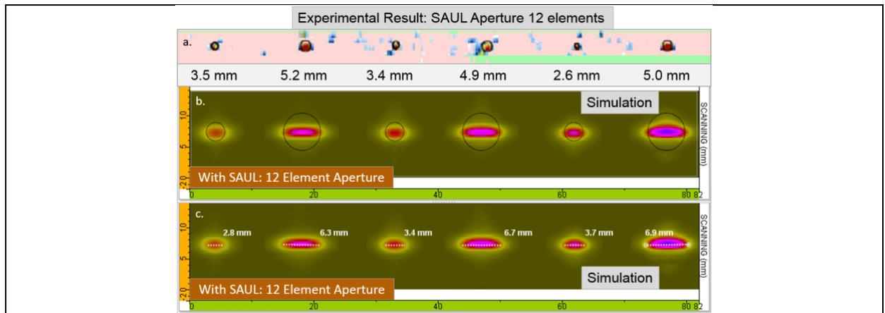
Figure 12. The top image (11a) shows the experimental C-scan for the convex radius measured using SAUL with a 12-element aperture. The estimated diameters are displayed below the image. The following two images show the same simulated C-scan obtained using SAUL also with a 12-element aperture. In Fig. 11b, black circles indicating the actual hole sizes are overlain on the C-scan. The bottom image (11c) shows the lines that were used to estimate the diameters of the indications.
