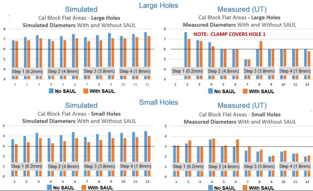
Figure 10. Holes sizes (diameters) are compared for simulated (left-hand side) versus measured UT images (right-hand side) obtained with and without SAUL (orange versus blue bars, respectively). The black horizontal lines in the charts indicate the actual hole sizes of 3 and 6 mm (confirmed by CMM measurements. **RENUMBER HOLES**)
