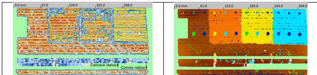
Fig. 8. Amplitude C-scan (left-hand image) and time-of-flight C-scan (right-hand image) for UT measurements on the composite calibration block for a SAUL aperture of 12 elements, with no focusing and a 25mm water path. The top images in each panel are scans of the flat sections. The radii scans were measured separately so that the scan plan and gain could be optimized for each region, but the gates were not optimized for imaging the holes.
